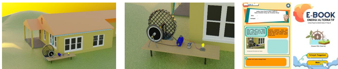
Figure 2. 3D interactive model of pico hydro rainwater system integrated within the e-book, illustrating energy conversion from harvested rainwater through turbine rotation to electricity generation
